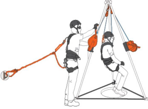
The best way to work in confined space is to use Tripods or Davit Arms. Retractable Fall Arrester easily installed on a Tripod can be used as a fall arrester when necessary or as a rescue device while operating manually. Retractable fall arresters with recovery mechanism are available in 9–42 metres. If secondary device is needed for safety, installation of a load winch is also possible.
