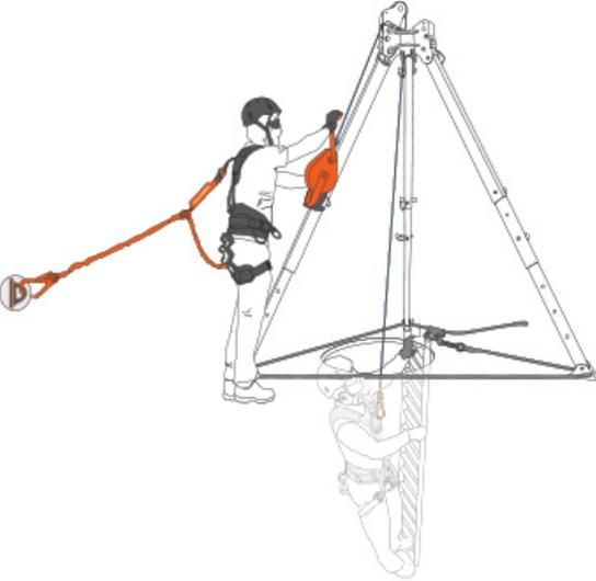
If there is a ladder in confined space the best way to work in there is to use a tripod with a Retractable Fall Arrester Block with Recovery Mechanism. Retractable Fall Arrester easily installed on a Tripod can be used as a fall arrester when necessary or as a rescue device while operating manually. Retractable fall arresters with recovery mechanism are available in 9–42 metres. If secondary device is needed for safety, installation of a load winch is also possible.
