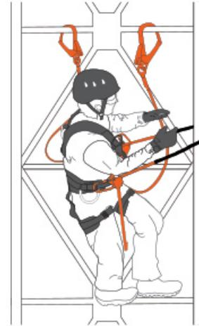
While working on a metal structured tower, using a double legged lanyard saves the user from a possible fall. Adjustable lanyards are designed to be used as part of a work positioning system and enable users to work at height in hands-free position. The lanyard is fitted around a supporting structure and then connected to the side D-rings on the operator's harness.
