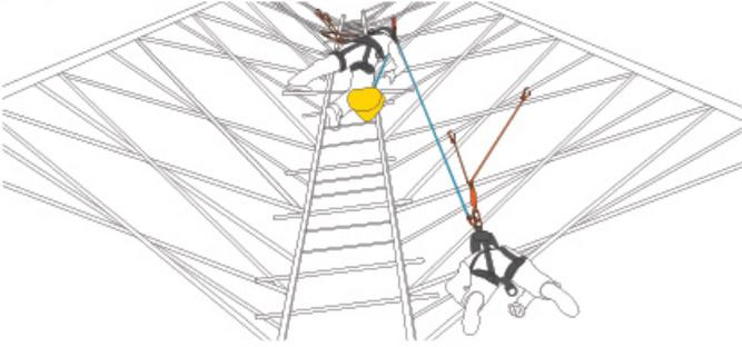
Suspended worker is lifted to higher position with rescue device to loosen the fall arrest lanyard.
