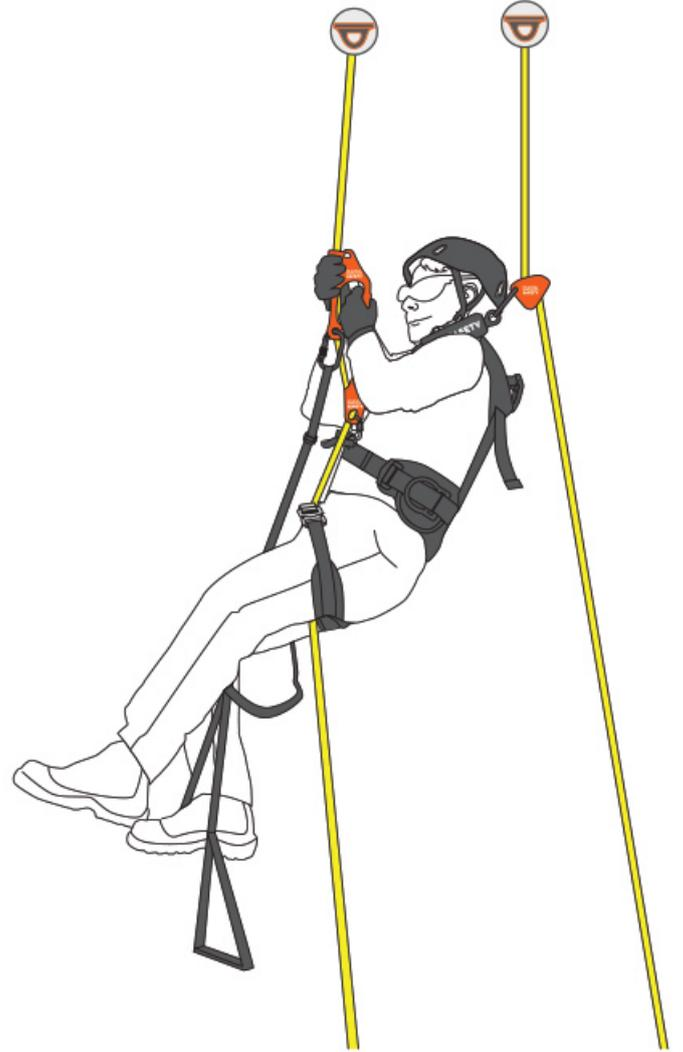
Ascender is used for ascending on the rope. Adjustable foot loops can also be used with handled ascenders.
