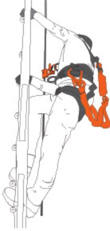
Monopole or Lattice towers are widely used in telecommunication sector. The safest way to climb up and down these towers is to use permanent vertical lifeline system installed on ladder (if such ladder exists). User is connected to the a vertical lifeline by a wire rope grab which is attached to the (A) chest attachment point of full body harness. When the user moves (up or down), it slides along the life line. In the event of a fall, the device stops the fall instantly on the cable.
