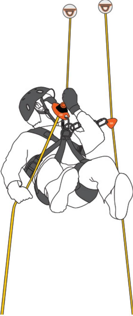
It is the most practical and fastest working technic to access working areas on a rope through a structure. A descender is placed on first rope and a fall arrester device with shock absorber is placed on second rope as back-up security.
