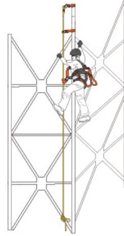
If there is no vertical lifeline fixed on tower, the first user who climbs up the tower with a double-legged shock absorbing lanyard creates a mobile vertical lifeline on tower using rope. The other users climb up the tower using this mobile vertical lifeline by the of appropriate rope grab. In case of a fall, the rope grab locks itself on the rope and stops the fall instantly.
