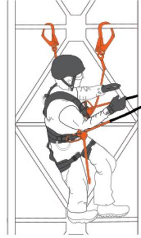
While working on a metal structured tower, using a double legged lanyard saves the user from a possible fall. Adjustable work positioning lanyards are designed to be used as part of a work positioning system and allow users to work hands-free position on these towers. The lanyard is fitted around a supporting structure and then connected to the side D-rings on the operator's harness.
