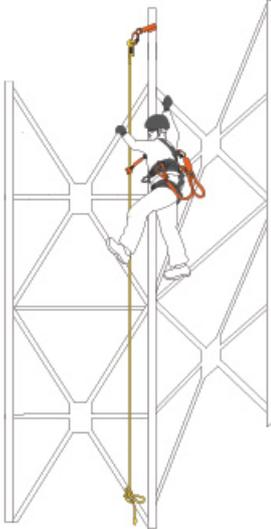
If there is no vertical lifeline fixed on energy towers, the first user who climbs up tower with a double-legged shock absorbing lanyard creates mobile vertical lifeline on tower using rope. The other users climb up the tower using this mobile vertical lifeline by help of appropriate rope grab. In case of a fall, the rope grab locks itself on the rope and stops the fall instantly.
