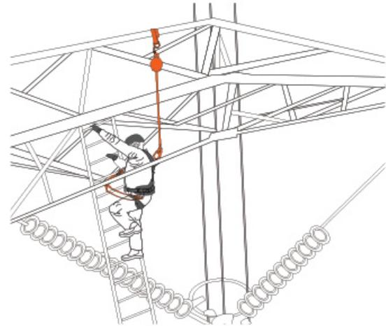
Use ladder to reach electrical insulators when working on electricity power lines. Retractable Fall Arrester Device should be used when moving up and down on ladders.
