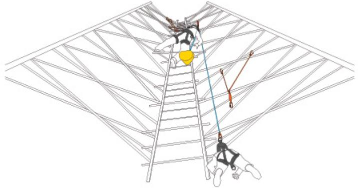
The suspended worker is lowered to the ground at a constant speed of 0.9 m/sec.
