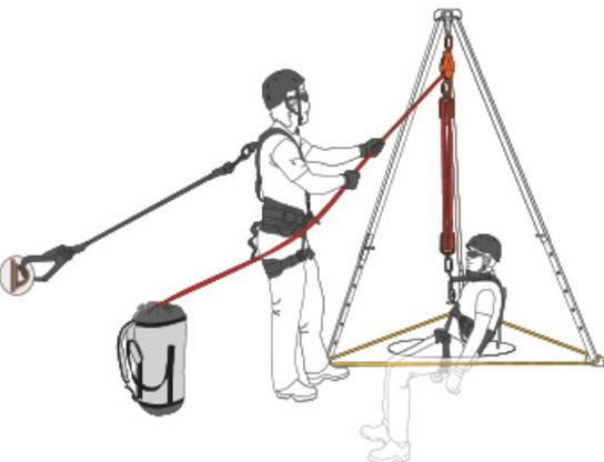
R-ALF rescue pulley is used as part of work suspension system in confined spaces as a user can easily lift/lower themselves. If the user loses control of the decent the over speed brake will automatically kick in. 11 mm static rope is recommended and the length of static rope depends on the depth of confined space and the pulley system to be used.
