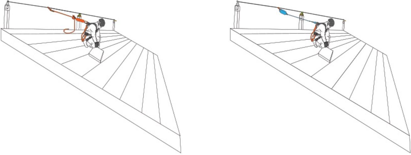
Fixed horizontal lifelines on the roofs that are installed by experts provides safety by creating continuous anchorage for the user along the lifeline. By connecting to the fixed lifeline with lanyard, slider, retractable fall arrester and rope fall arrest system, user ensures the safety against possible fall.
