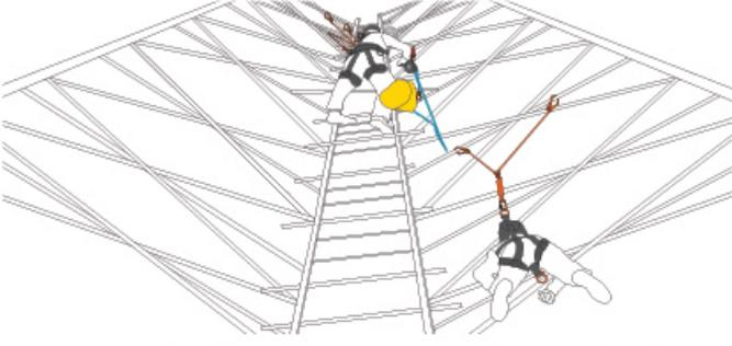
Rescuer attaches himself to a secure anchorage point located above suspended worker with ABS 3WH rescue device.
