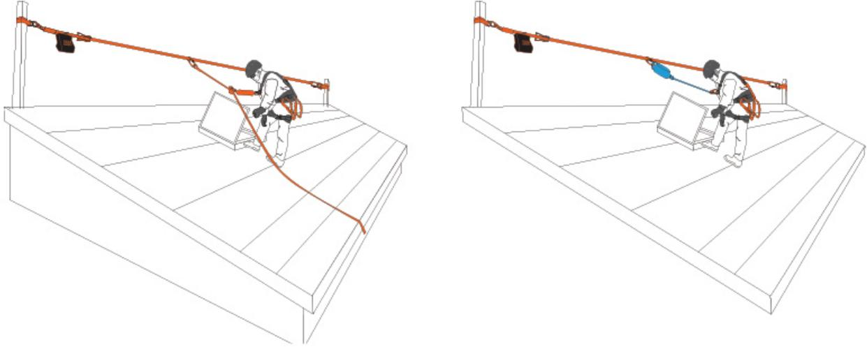
If there is no permanent lifeline system on the roof then mobile lifeline system must be installed for safe work to be performed. This system must be installed by competent person who has the necessary technical skills and training. NOTE: USER QUANTITY DEPENDS ON THE PRODUCT. MAX USER QUANTITY CANNOT EXCEED THE NUMBER THAT MANUFACTURER INDICATES.
