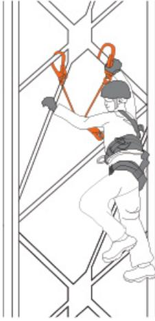
If there is no vertical lifeline fixed on energy towers then user uses the double-legged shock absorbing lanyard to move around the tower whilst being connected at all times. It is recommended the fall arrest and positioning harness to be conforming EN358-EN361-EN 813 standards and to attach double-legged shock absorbing lanyard to the (A) chest attachment point of full body harness.
