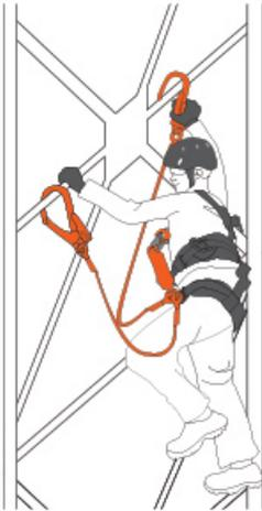
If there is no vertical lifeline fixed on towers then user uses the double-legged shock absorbing lanyard to move around the tower whilst being connected at all times. It is recommended to attach double-legged shock absorbing lanyard to the (A) chest attachment point of full body harness
